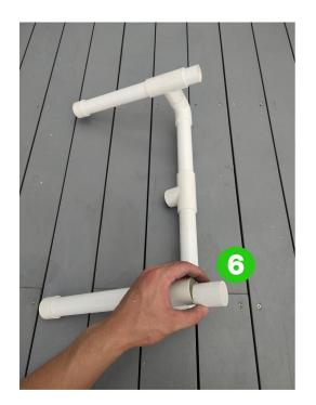
Insert No. 6 into No. 12, making sure the height is the same on both sides
