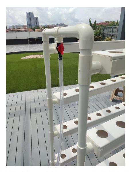
No14 (Flexible conduit) connect to No15 (Valve) and then connect to No 13
