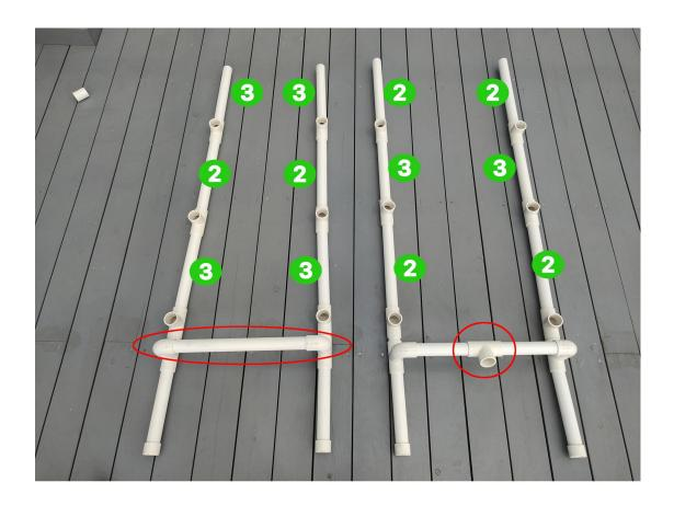
As shown in the figure, install the pipes with the corresponding specifications in order to ensure that the installation direction is correct and the height is consistent.
